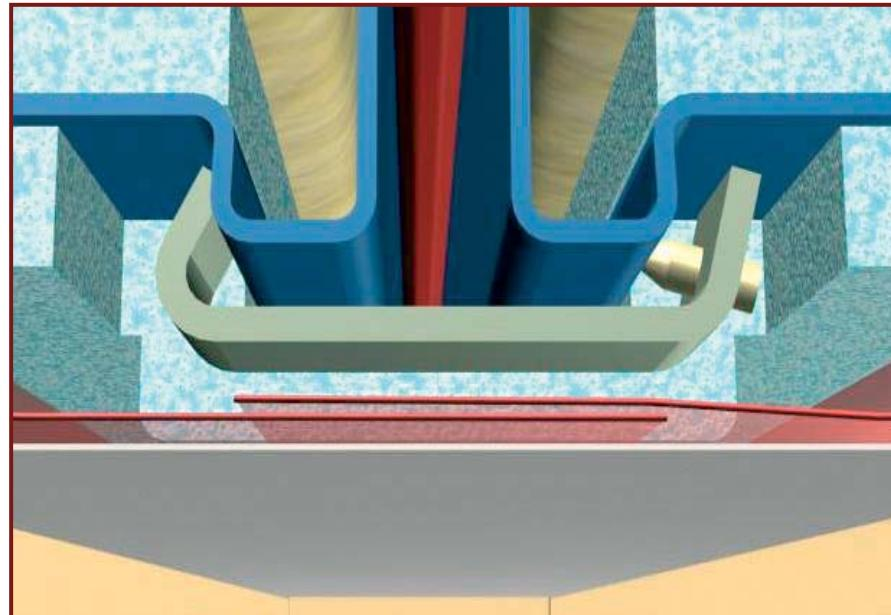
**EN:** Cut out the styrofoam with a knife at the areas where the internal clamps are fitted. Bolt together both corner posts with internal clamps. Overlap and stick together the vapour barriers (folis) continuously by using an adhesive tape.
