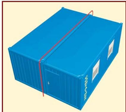
**EN:** The single units have to be placed side by side (end to end) with a distance of approx. 20 mm in between.
