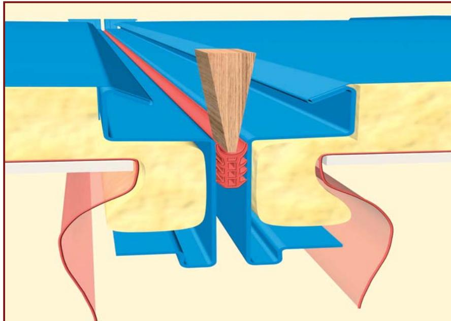
**EN:** Insert the special rubber seal between the cabin frames and drive it in with a wedge.
