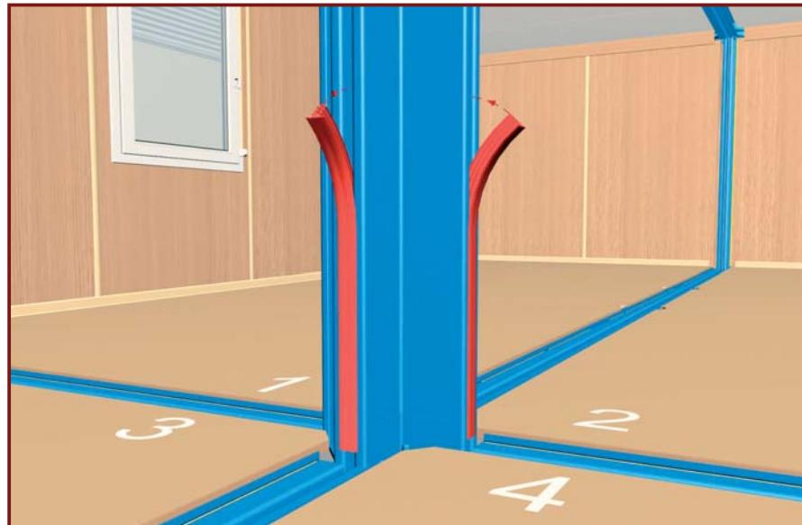
**EN:** Cover the internal gaps with the remaining rubber seal.
